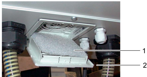
Fig. 5-8: Exchanging the lower filter mat
