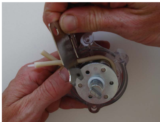
Fig. 5-19: Removing the mounting aid
