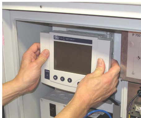
Fig. 4-6: IQ SENSORNET terminal
