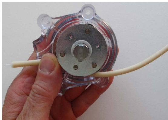
Fig. 5-16: Inserting the tube in the dent
