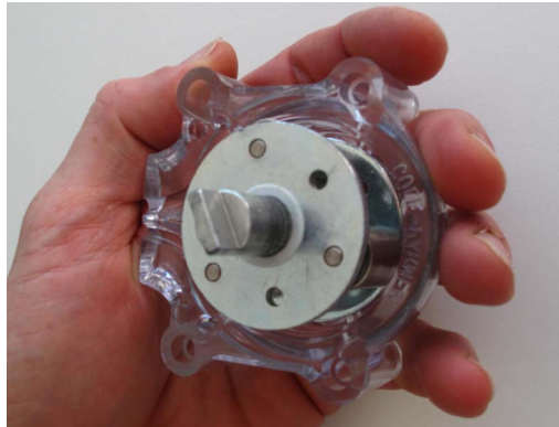
Fig. 5-14: Holding one half of the pump head (tube openings are on the left side)
